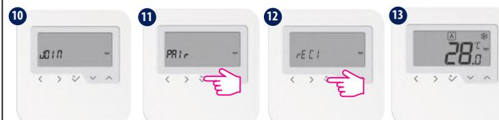
For pairing with RX2, set the internal switch of the receiver to RX2 and choose **r-E C2** at step 4. After that, follow the same procedure as described above.
