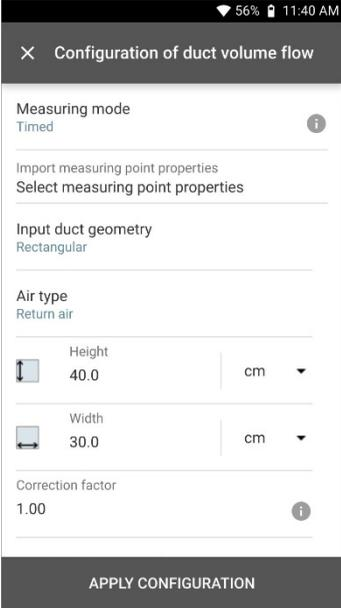
Configuration of duct volume flow
